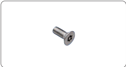
item no.: Z070 special countersink tamper-resistant screw M6 x 16, V2A, for clamp fixtures, similar to DIN7991
