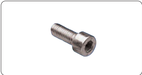
item no.: Z098-VA cylinder head screw DIN912 - M8 x 20 for 4831/32/36/37
