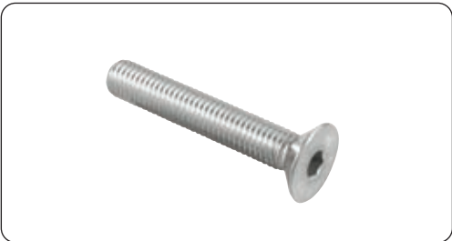
item no.: S7991A2D countersink screw DIN7991 - M10 x 45/60 S7991A2D10X45 S7991A2D10X60
